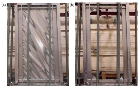
Figure 6. Tension field during testing : (a) Test specimen W35 (b) Test specimen W35F
