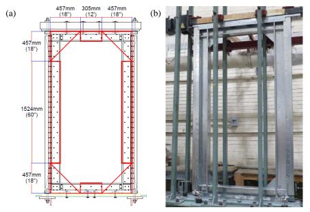
Figure 5. Frame-only shear wall W37F: (a) configuration and dimensions, (b) specimen installed in test frame
