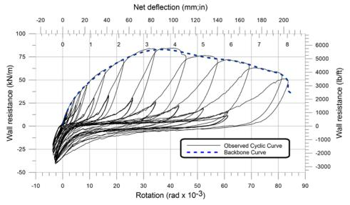
Figure 8. Conversion of W37 force vs. deformation hysteresis to a backbone curve
