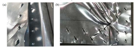
Figure 2. (a) Bearing of exterior sheathing resulting in pullover, (b) bearing of interior confined sheathing (Santos [4])
