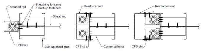
Figure 3. Left to right : no reinforcement, R2, and R3 reinforcement schemes for the chord stud members
