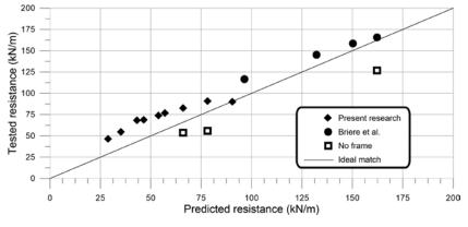
Figure 9. MESM S<sub>u</sub> prediction versus tested results
