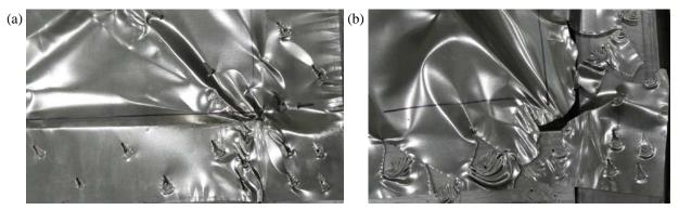
Figure 7. Bearing damage : (a) Specimen W36, (b) Specimen W37 with torn corner due to extensive drift demand
