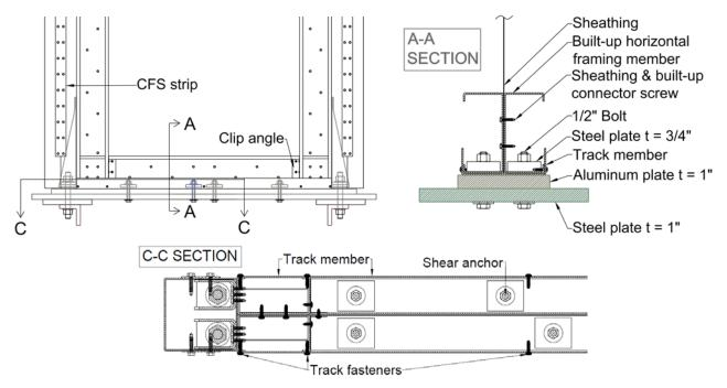
Figure 4. Detailing of centre-sheathed shear wall
