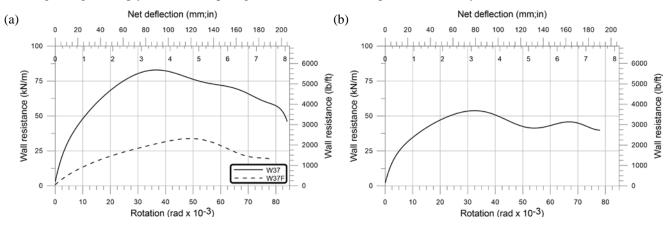
Figure 10. W37 force vs. deformation : (a) full wall and frame-only, (b) Difference between the two backbone curves
