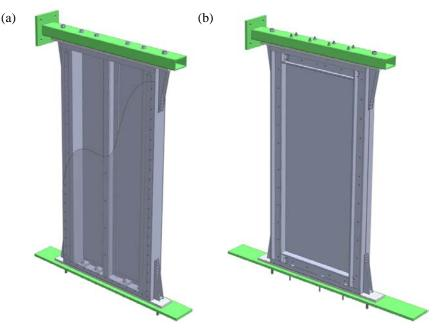
Figure 1. CFS shear walls : (a) double-sheathed configuration with cutaway view, (b) centre-sheathed configuration
